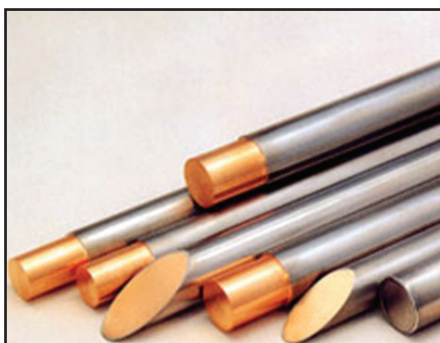
Fig 3.16: Diffusion bonded parts manufactured via HIP process (courtesy of MTC)
