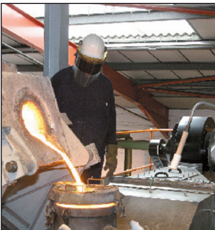
Fig 3.3: Pouring melt into atomiser (courtesy of Atomising Systems)
