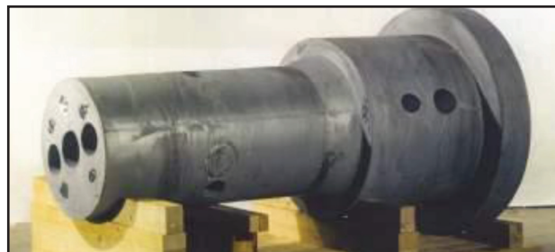
Large nine tonne stainless Near Net Shape part for oil and gas industry (courtesy of Sandvik Powdermet)
