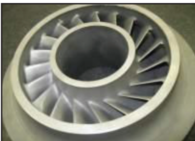
Net Shape Nickel-base impeller for gas compressor (courtesy of Syntertech)
