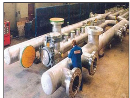
Fig 3.18: Manifold with 1-7 tonnes sections assembled by welding (courtesy of Sandvik Powdermet AB)
