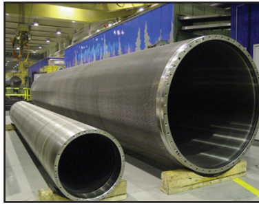
Suction roll shell for paper machines (courtesy of Metso)
