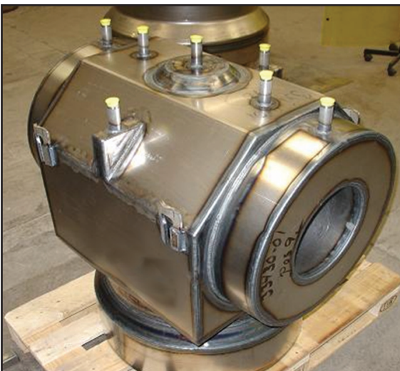
Fig 3.11: Example of container construction with filling / evacuation tubes (courtesy of Rolls Royce.)
