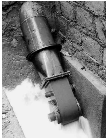
Fig. 13. Low cost crossflow turbine in India. This 5 kW machine, designed and disseminated by IT Power of the UK, is used for rice-hulling and electricity generation.
