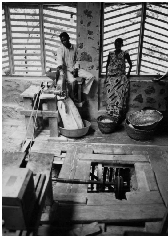
Figure 2. Interior of turbine house with flour mill. Photograph by author, near Boyangana, 1995
