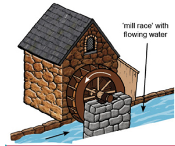
Figure 2-5 Undershot water wheel
