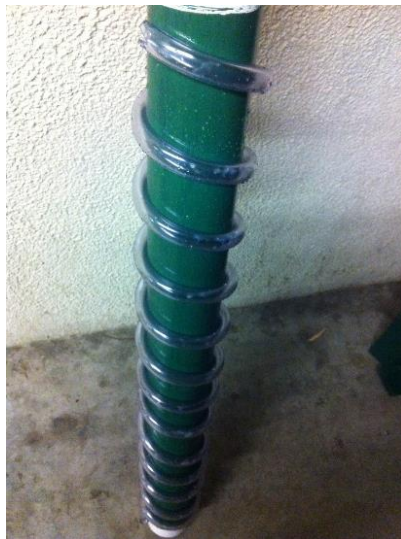
Figure 5-6 the vinyl tubing wrapped around the pipe to create an "Inside out Screw"
