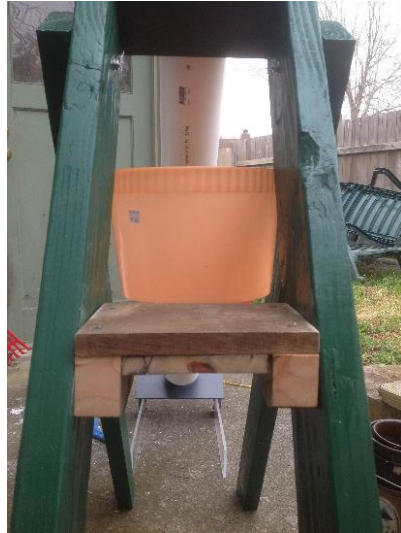
Figure 5-4 the terminal reservoir to catch pumped water
