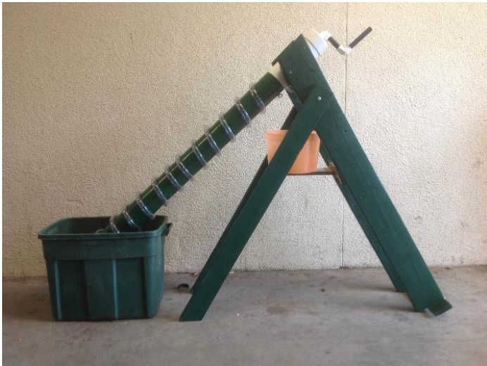
Figure 5-1 the completed Archimedes Screw Pump
