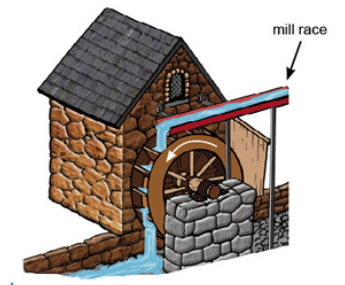
Figure 2-6 Overshot water wheel
