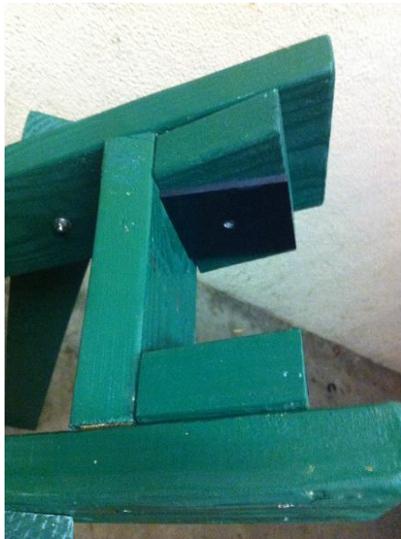
Figure 5-11 the slot on the Stand to support the Archimedes Screw Pump during rotation
