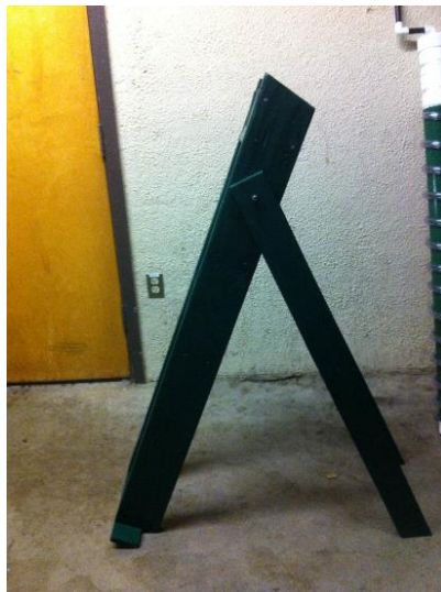
Figure 5-10 the stand of the Archimedes Screw Pump for set up
