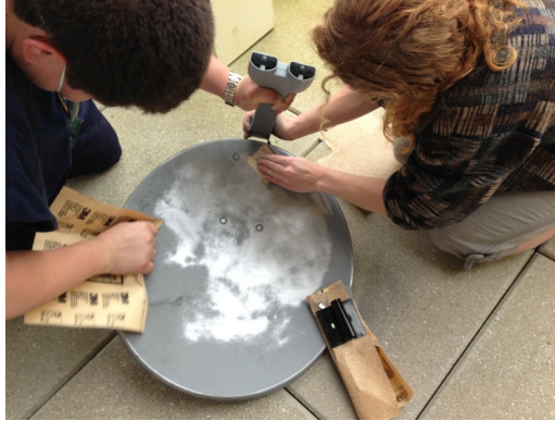
Figure 5-5 Josh Martinez and Mary Krieger sanding the satellite dish. Surface was sanded by hand due to the concave shape of the dish.
