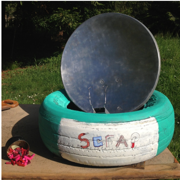
Figure 5-1 Completed Solar Heater with assorted crayons to be melted. Sun is reflected off the dish and focused down on to the vessel containing wax.
