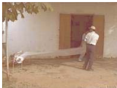
Photo 6. Putting a steel rod (or bamboo pole) through the centre of the roll facilitates the extraction of the required length of tube
