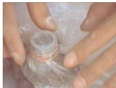
Photo 26. Covering the gas outlet with a plastic bag
