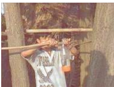
Photo 49. Suspending the water trap
