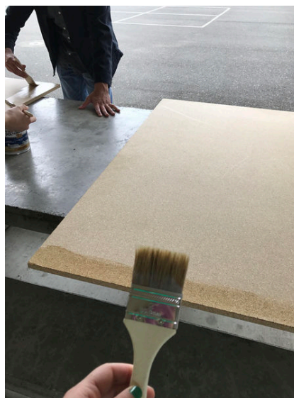
Figure 5-10: Finishing particleboard shelving with polyurethane. Image taken by Haley Isaacson on 4/17/17.
