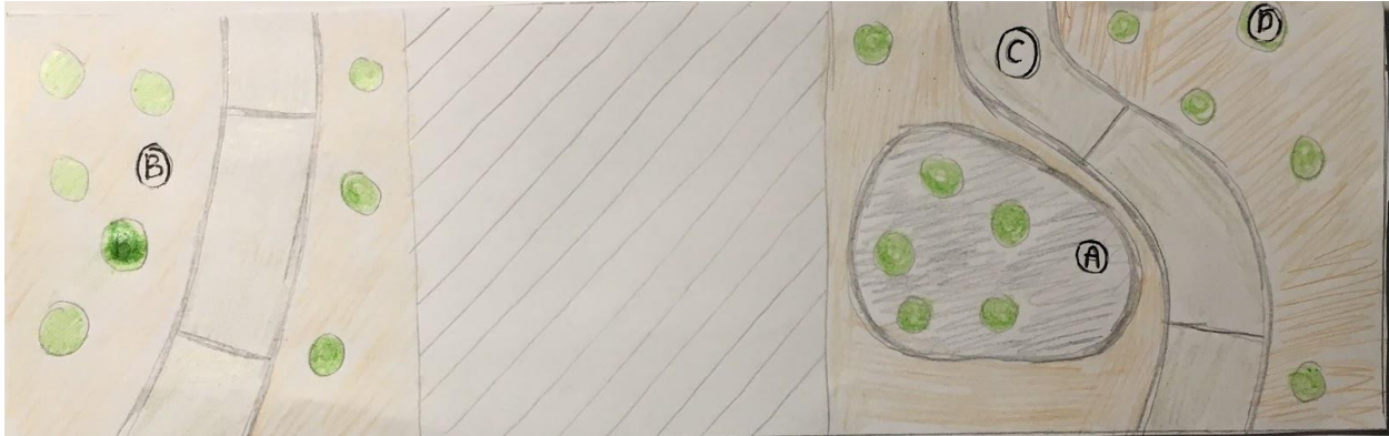
Figure 3-4: Xeriscaped Rectangle is made up of semi permeable cement paths (C) like the ones used in front of the school. Drought tolerant plants shown by (D) would grow in soil or possibly mulch (B). A circular section, contained by a short wooden barrier (A) contains gravel and more drought tolerant plants to give the alternative a visual appeal.
