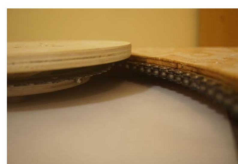
D: Bike Chain lining the circumference of the plywood top piece.
