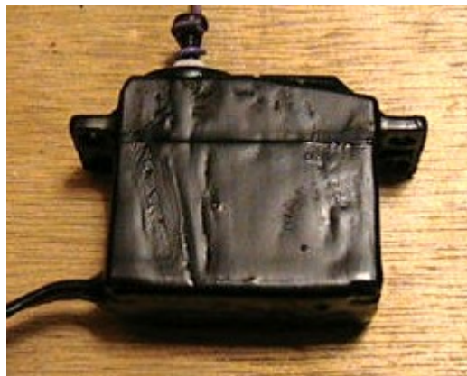
Figure 2-25: Waterproofing by coating in plastic (Society of Robots 2012).
