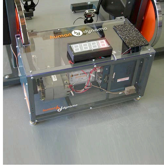
Figure 2-22: Four parallel exercise generators and communal battery pack (Human Dynamo 2011).
