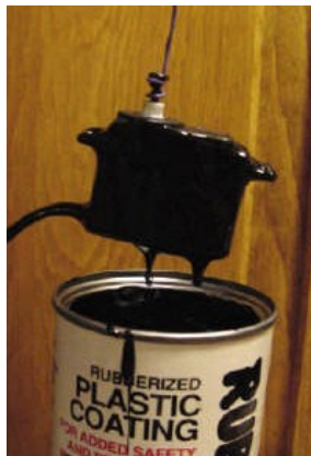
Figure 2-25: Waterproofing by coating in plastic (Society of Robots 2012).
