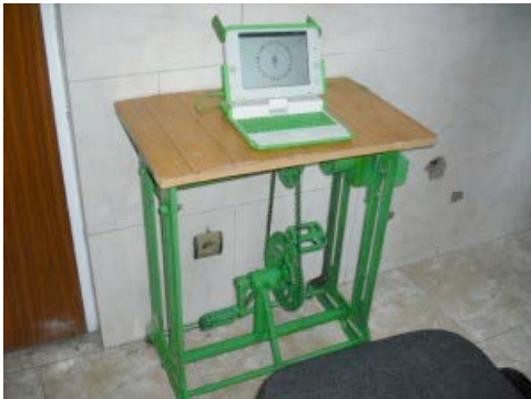
Figure 2-23: Pedal powered laptop (left, OLPC Afghanistan 2011), and a pedal powered washing machine (right, Pilloton 2007).
