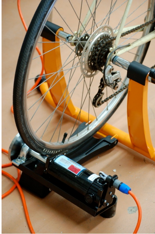
Figure 2-19: Basic bicycle power generator (Airstream Life 2008).
