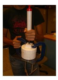
We then pumped the chamber up as high as we could. After we detected air loss as the pressure was dropping at pressures greater than 40 psi, we filled the test chamber with water to observe where the leakage was occurring.
