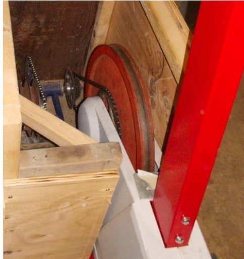
Figure 5-5 Bicycle Chain Drive connected to Intermediate Shaft
