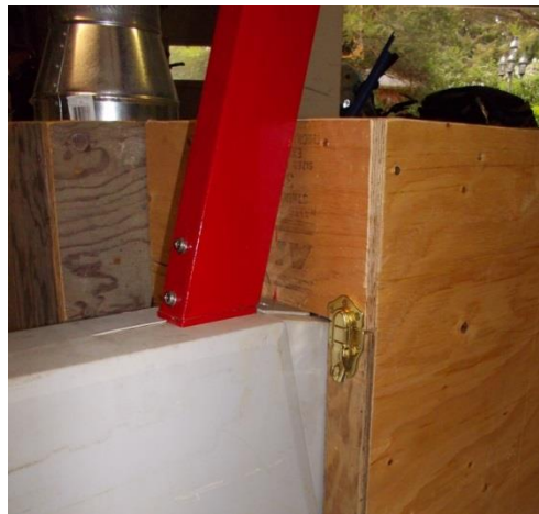
Figure 5-6 Drive Component Shield, secured
