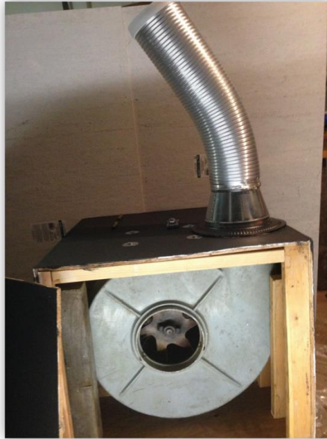
Figure 5-7 Attaching Discharge Nozzle to Blower Box
