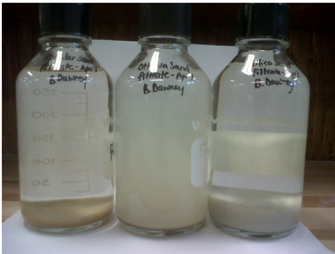
Figure 4 - Settled effluent after 1 day. Effluents are from regular sand (left), Ottawa sand (center), silica sand (right).
