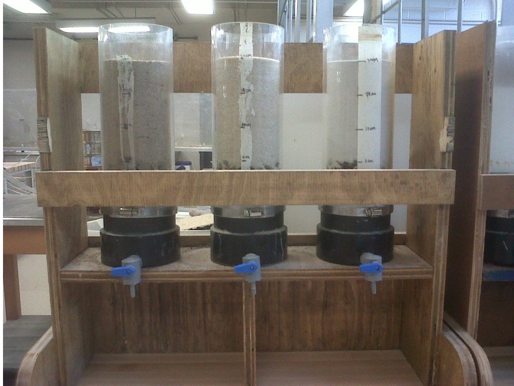
Figure 2 - Prepared filter columns: regular sand (left), Ottawa sand (center), silica sand (right).
