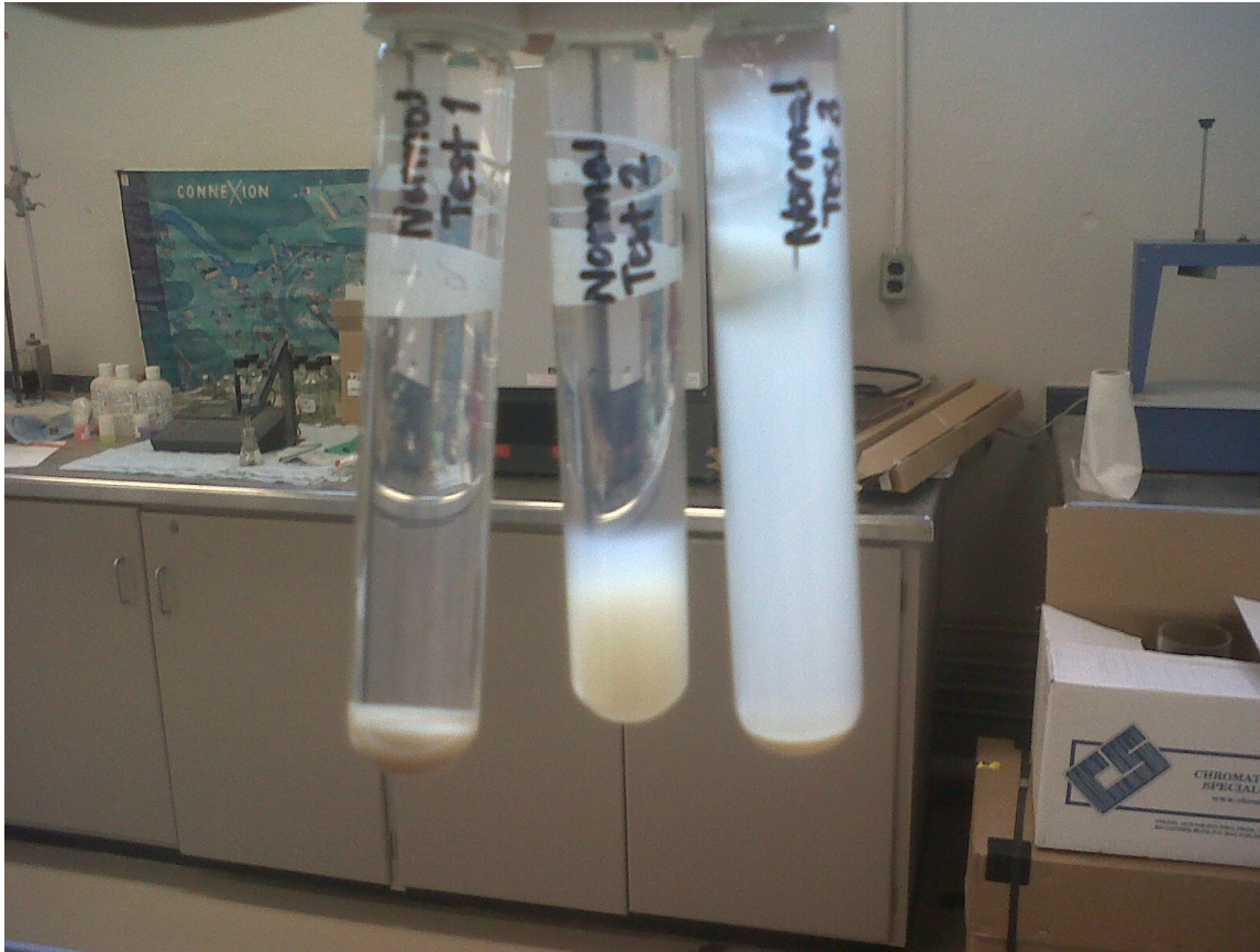
Figure 6 - Settling observed after one day in a sample of the collected filtrate from the regular sand filter. The differences in Trial 1 (left), Trial 2 (center) and Trial 3 (right) illustrate how settling occurred optimally when there were a relatively high amount of fines that passed through the filter with the sample turbid water (Trial 1).
