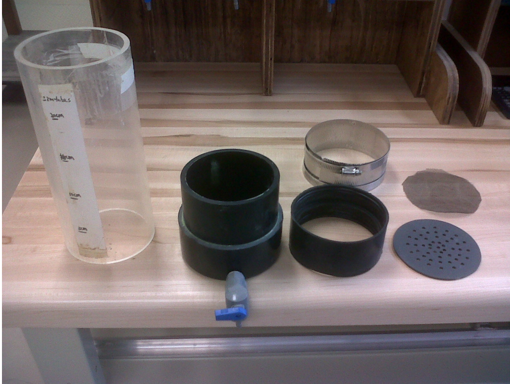
Figure 1 - Components of a filter column.
