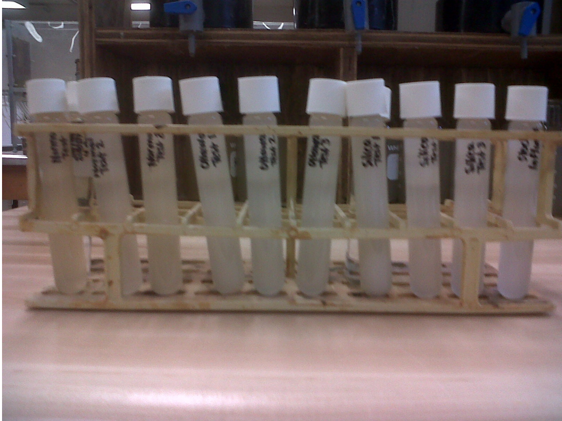
Figure 5 - Unsettled effluent from each of the filters. From left to right, 1-3 are regular sand effluent; 4-6 are Ottawa sand effluent; 7-9 are silica sand effluent; and 10 is stock influent for baseline comparison.
