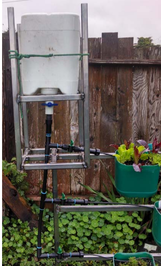
Figure 5-5: The reservoir tank dispenses water to the main 1/2 inch tubing line of the irrigation system.
