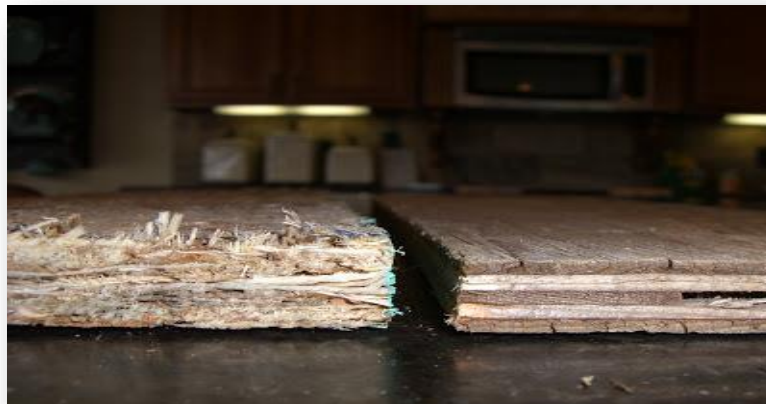
Figure 2.7 The difference between OSB and Plywood (Lumber and Plywood 1998)
