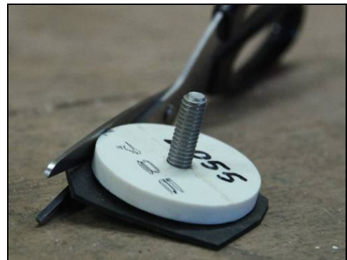
Rubber disc being cut on template
