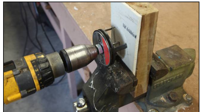
Hole Sawing using a hand drill
