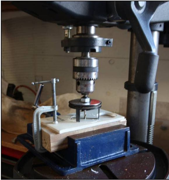
Hole Sawing using a drill press
