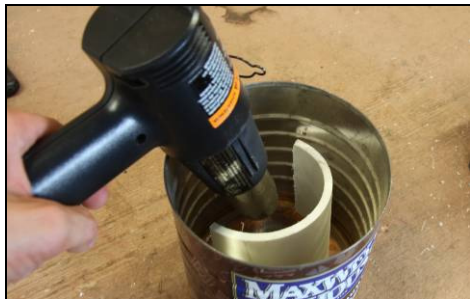
Heating PVC with an electric heat gun
