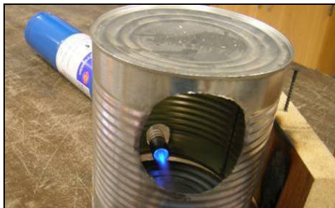
Heating PVC with a torch
