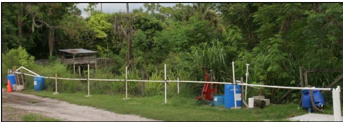
Rower pump with 60' horizontal run from borehole
