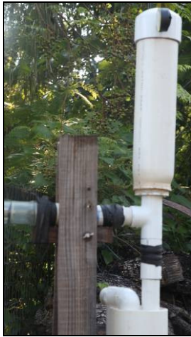
Surge chamber on rower pump
