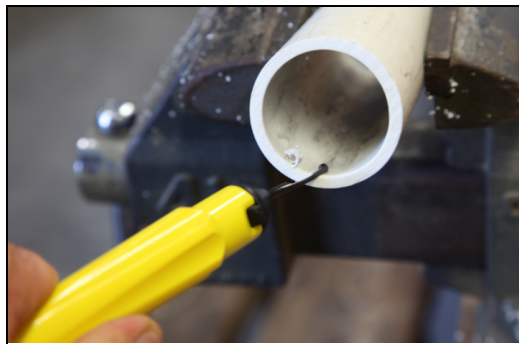
Deburring tool removing burrs on inside edge of pipe
