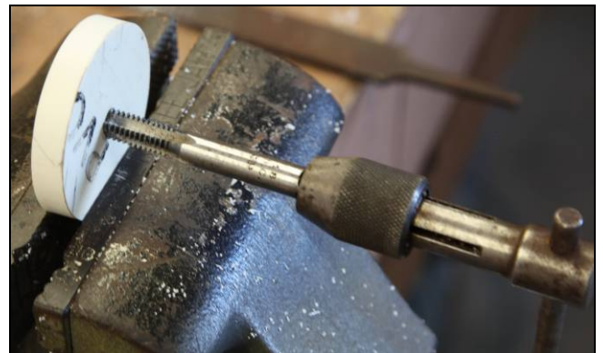
Tapping threads in a PVC disc.
