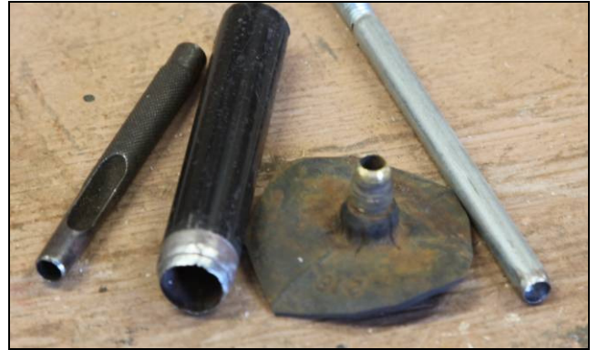
From left to right: standard circular punch, metal pipe sharpened to a cutting edge, valve stem sharpened to a cutting edge, drilled-out metal stock sharpened to a cutting edge.
