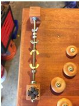
Fig 7: This metal bar contains nuts and wingnuts that can be twisted the entire span of the metal rod. There is also buttons taken from a video game controller on top of one of the wooden blocks
