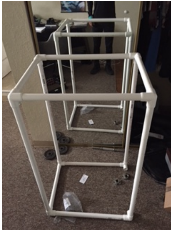
Figure 5-7: Assembled PVC frame (I. Duque, unpublished photos, April 2018)
