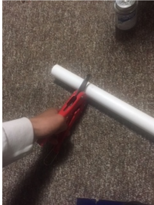
Figure 5-6: Cutting the PVC pipe to size (I. Duque, unpublished photos, April 2018)
