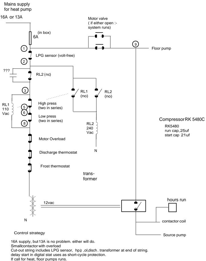
Floor pump or source pump run-on not thought necessary
