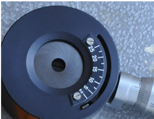
Figure 2-4: An image of a lens aperture in its smallest diameter (Nave 2017)
