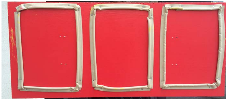
Figure 5.2.7: Shows the three separate fitted seals for each sink.
