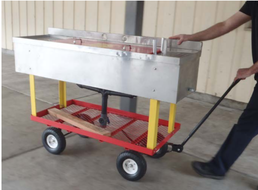
Figure 5.2.3: Cart being transported with wagon style steering.
