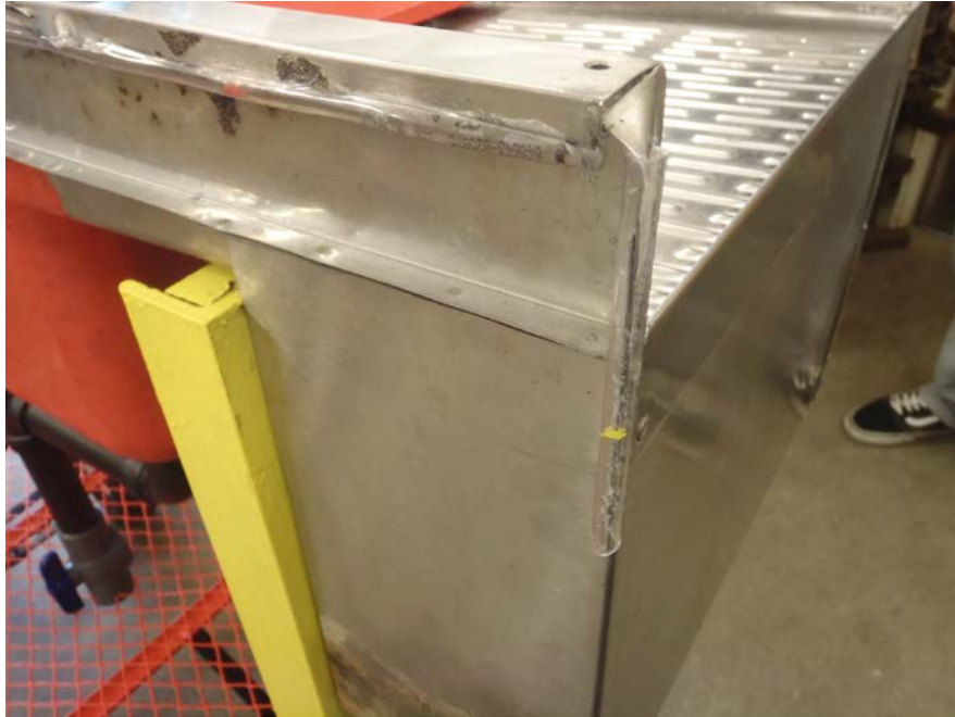
Figure 5.2.10: Plastic tubing is used to cover the sharp edges of the sink.
