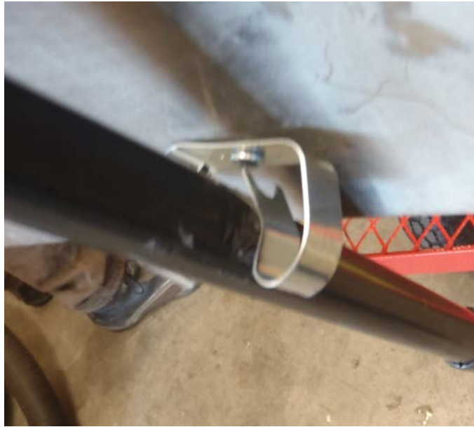
Figure 5.2.8: An image of the tension clip in use holding up the steering handle.
