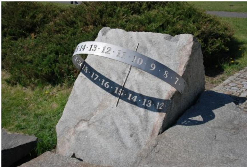
Figure 2.7 Strip type equatorial sundial (Zorro 2011)
