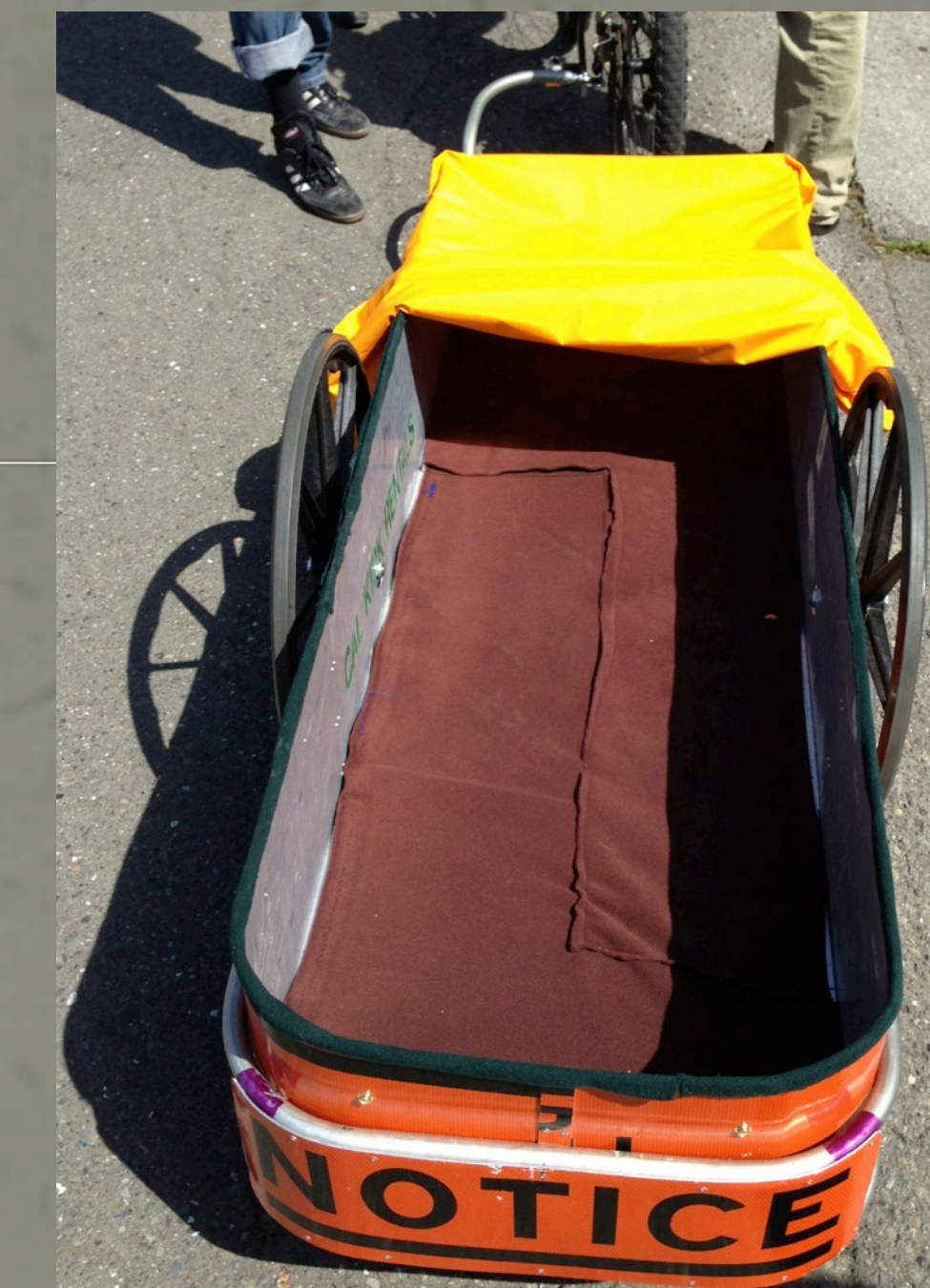
Lined with felt to minimize noise from loose goods
