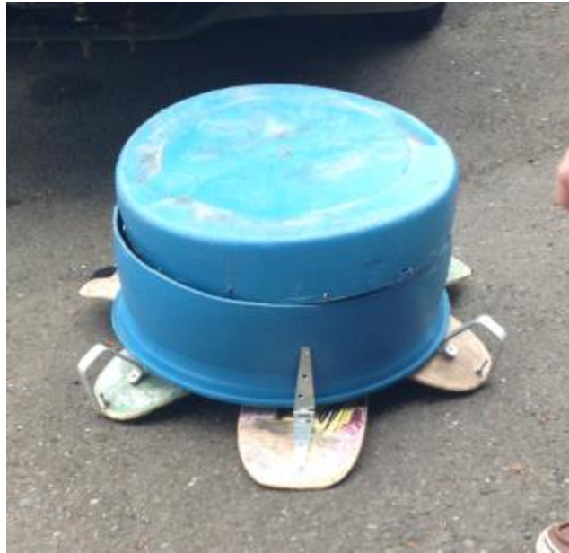
Figure 5-5: Completely collapsed basket
