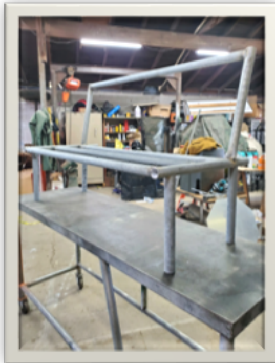
Figure 57 The galvanized steel frame. By Hayden Miller.
