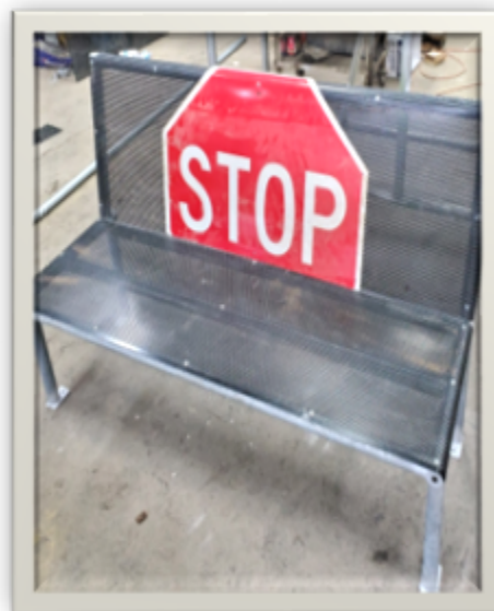
Figure 510 Adding signs onto the perforated metal on the bench frame. By Hayden Miller.
