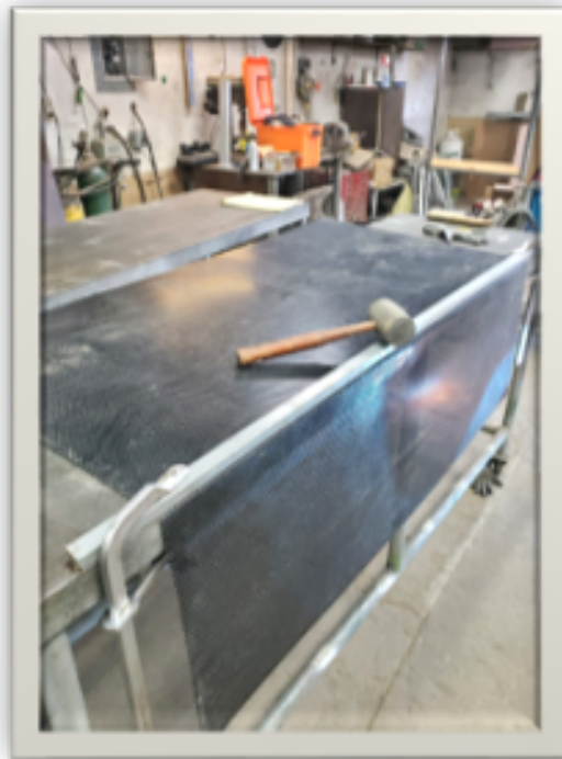
Figure 58 Bending perforated metal around the frame. By Hayden Miller.
