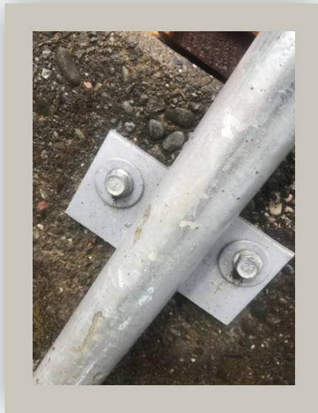
Figure 511 Welded flange prototype used to test function, sturdiness, and durability.
