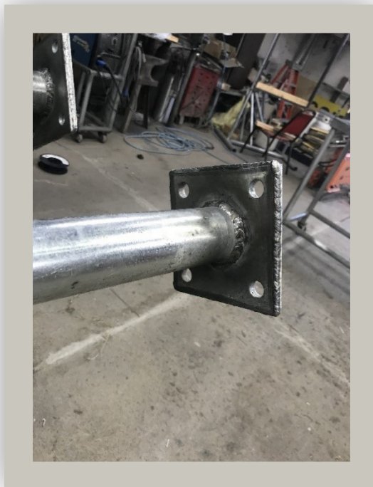
Figure 512 Another flange prototype. By Hayden Miller.
