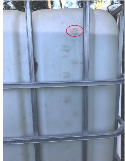
Figure C-4. Tank at full capacity 1000-liter (264 gallons)
