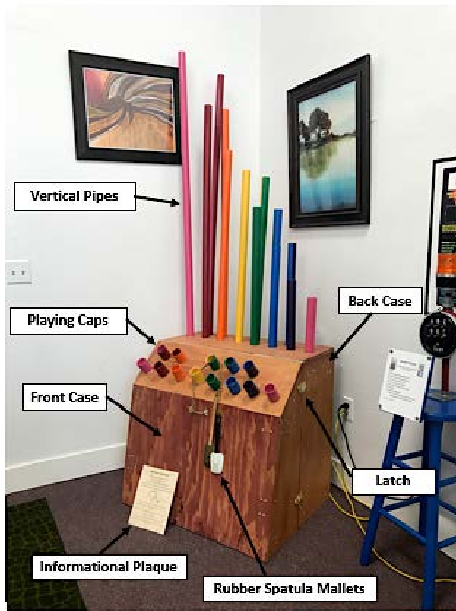
Figure 5-1: The Sound Garden. The assembly contains the front case, the back case, the elbow assembly (not pictured), the playing caps, the vertical tubes, two rubber spatula mallets, latches, and an informational placard.
