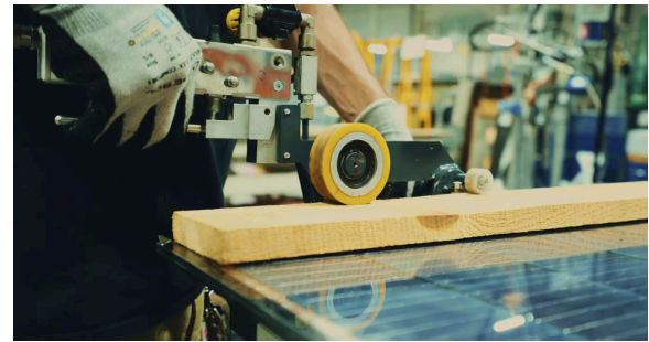
Figure 7. Semi-manual sealing of edge-sealant
