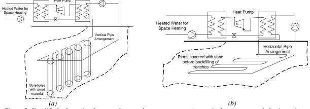
Figure 2. Simplified schematic of a ground-source heat pump system (a. vertical arrangement, b. horizontal arrangement) shown here configured for a hydronic space heating application.
