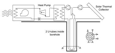
Figure 7. Simplified schematic of the 2 U-tube configuration proposed by Bernier and Shirazi (2007)
