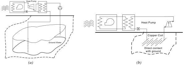
Figure 3. Simplified schematic of a ground-source heat pump system (a. open loop, b. direct exchange) shown here for air space heating
