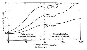
Figure 5. Annual solar fraction as a function of storage capacity of water tanks for three collector areas based on Madison meteorological data (Duffie and Beckman, 2006).
