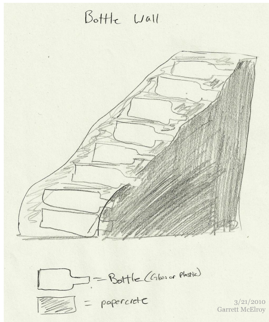
Figure 3.2- 9: This diagram shows a birds-eye view of a cross section of the bottle wall.
