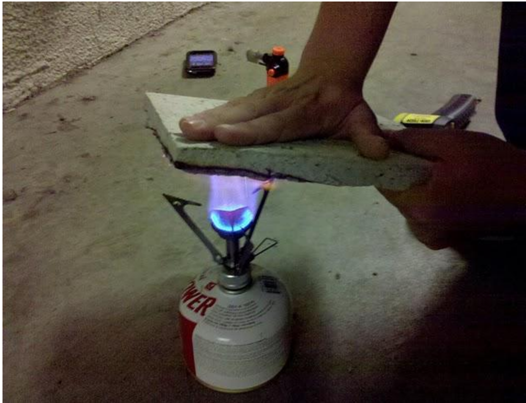
Figure 5-7: The side of the sample unexposed to heat remained cool during heating (Thompson, 2010).
