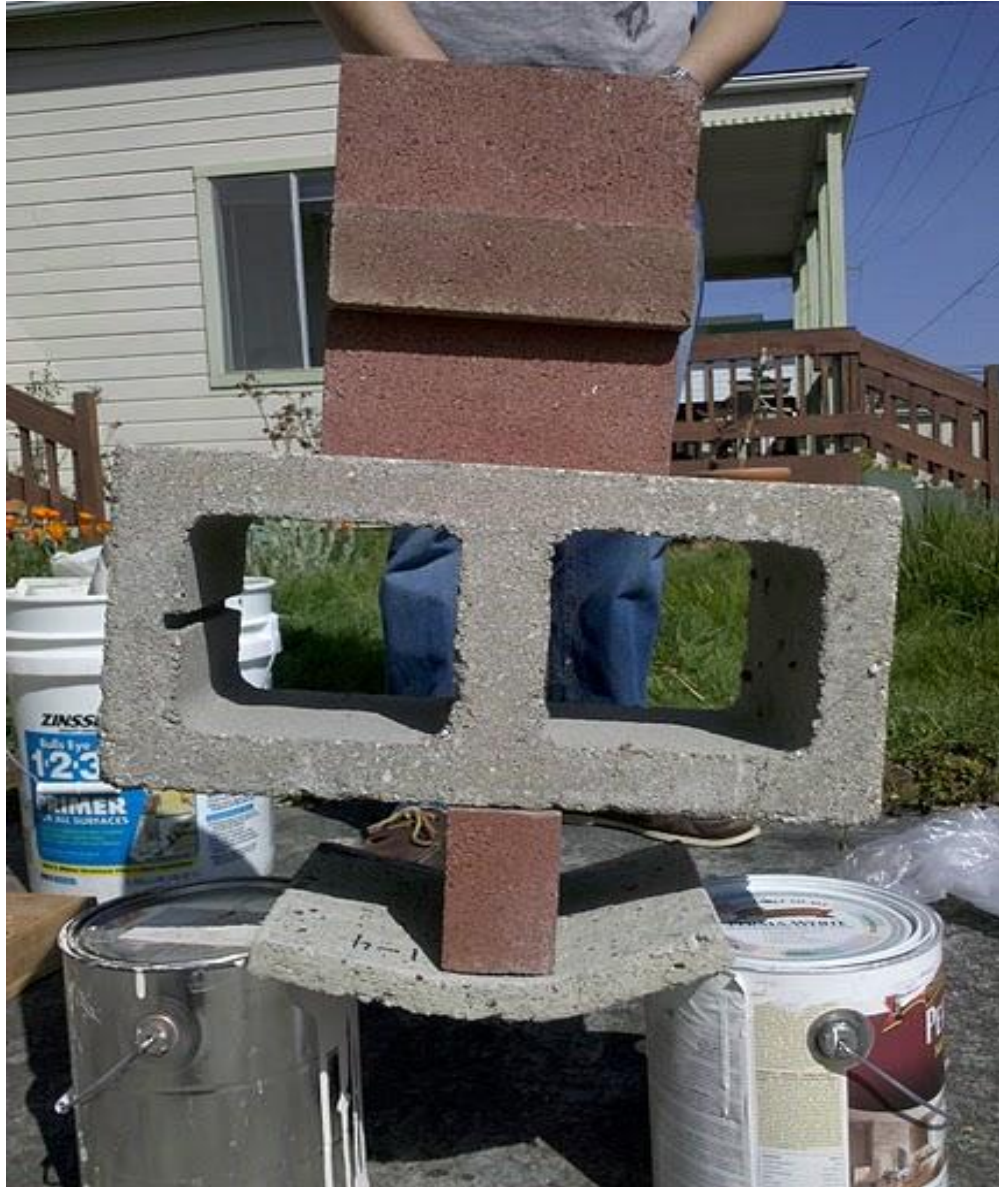
Figure 5-8: The Papercrete model suspended on paint cans supported a fifty pound load (Williams, 2010).
