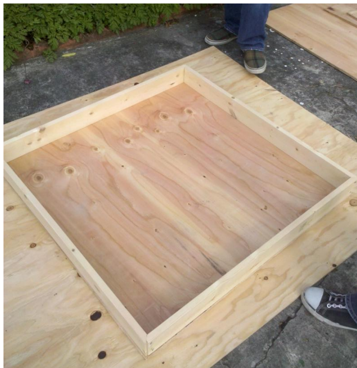
Figure 5 - 2: The end product of the frame. This frame is 3 ft x 3 ft and 3 inches deep (Williams, 2010).
