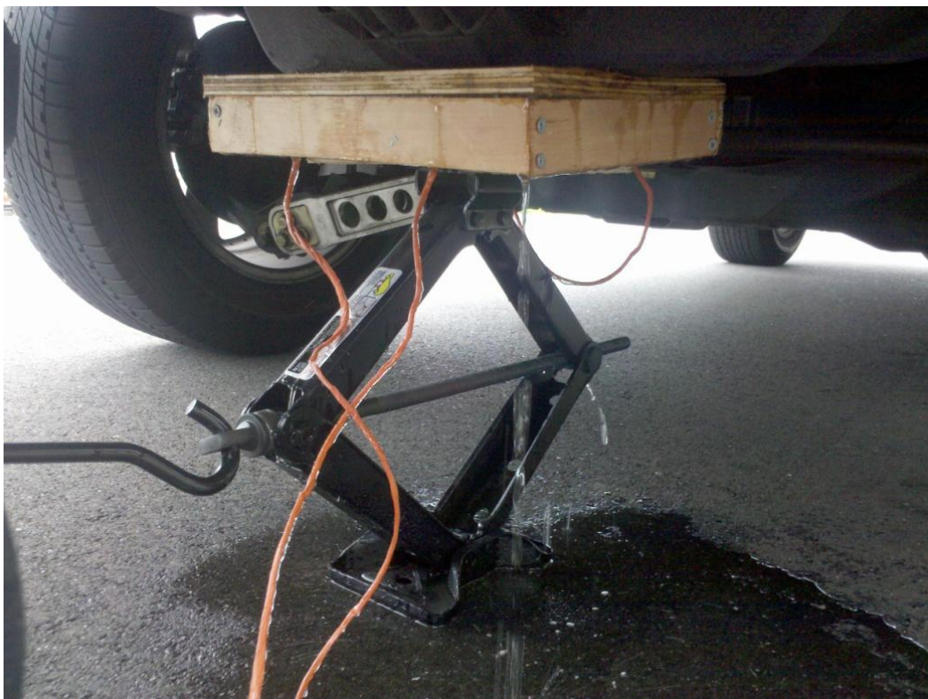
Figure 5–4: The weight of the car compresses the mold and drains all of the excess water (Williams, 2010).
