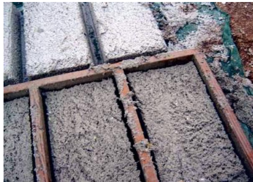
Figure 2.3-3: Papercrete blocks are drying in the mold (Sanders, 2009).
