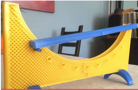
Figure 2-3: Brachistochrone device made by a 3D printer design. Open source CAD design from Makerbot's Thingiverse online community.
