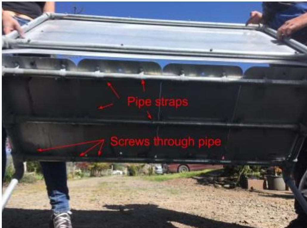
Figure 5-10: Underside of larger bench.
