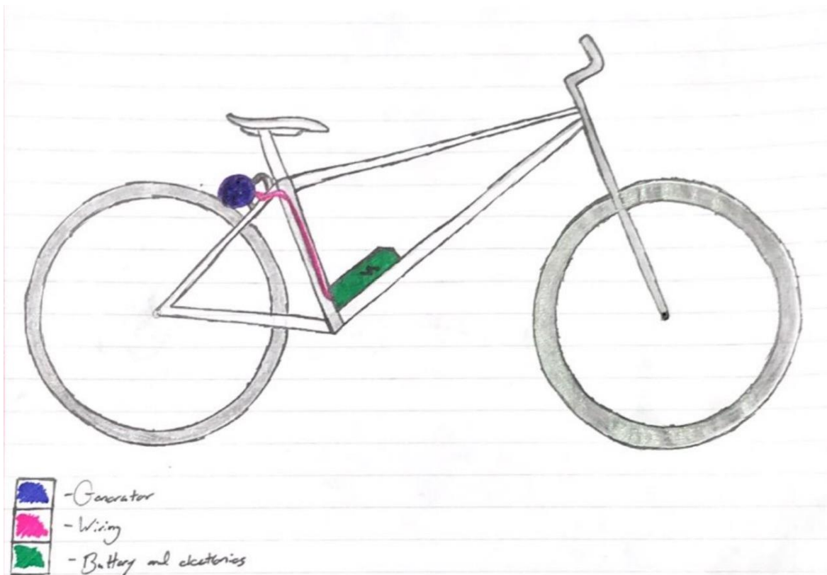
Figure 3-2 Drawing of V1 Attachable Friction Motor
