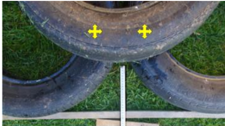
Figure 5-10 Placement of second row of tires.
