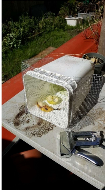
Figure 5-22. The device used to prototype the quality of pest-resistant of the hardware cloth. By Kelsey Burrell.
