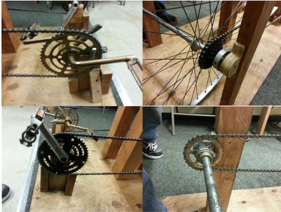
Figure 5-4 Chain and crank shaft system that rotates the wheel.
