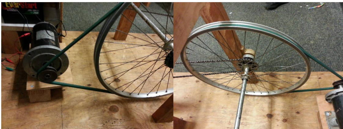
Figure 5-5 Pulley system driving the generator.
