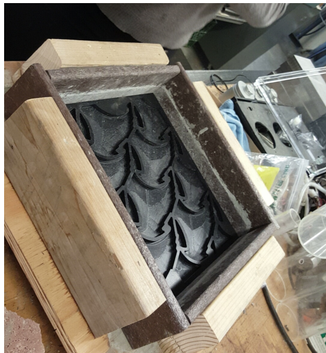
Figure 28 Finalized Form with Plastic Mold Addition
