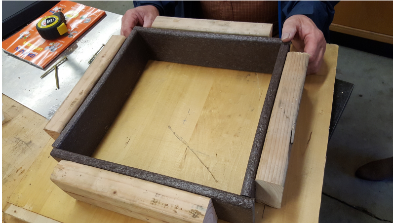
Figure 27 Finalized Concrete Pouring Form
