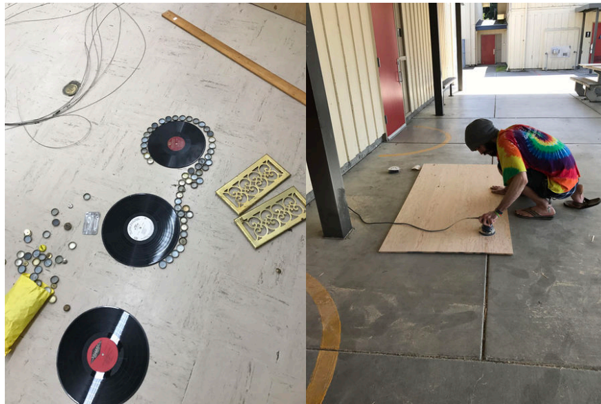
Figure 5-11: Laying out violin design for side panels (left). Sanding CDX plywood used for side panels (right). Images taken by Haley Isaacson on 4/17/17 and 4/21/17 respectively.
