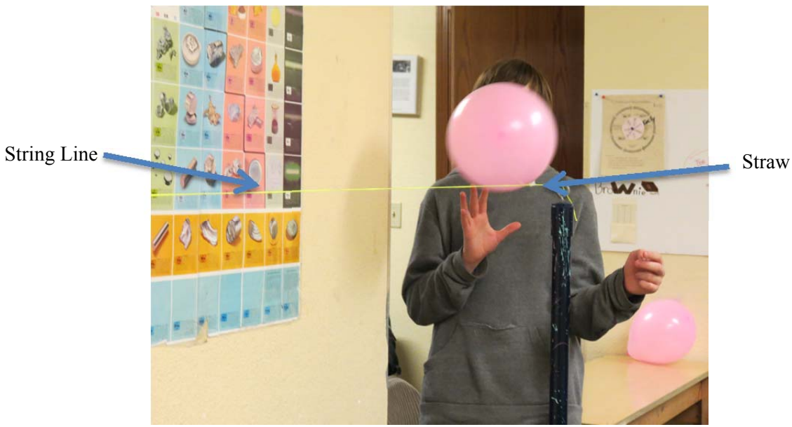
Figure 5-7: How the balloon is attached to the string (2012, C. Alston)
