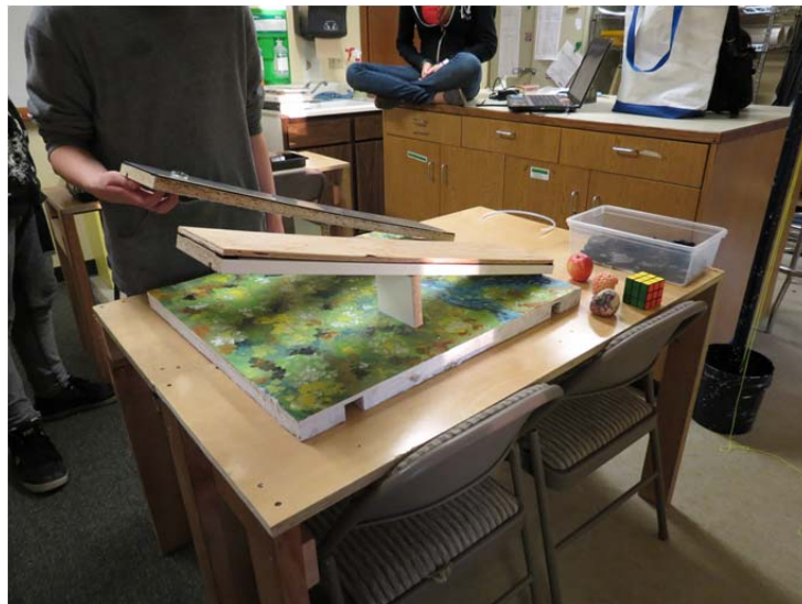
Figure 5-3: Adjustable angles allow students to change the planes. (2012, C. Alston)
