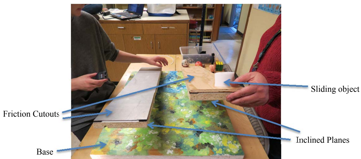
Figure 5-1: Inclined Planes apparatus in use. (2012, C. Alston)
