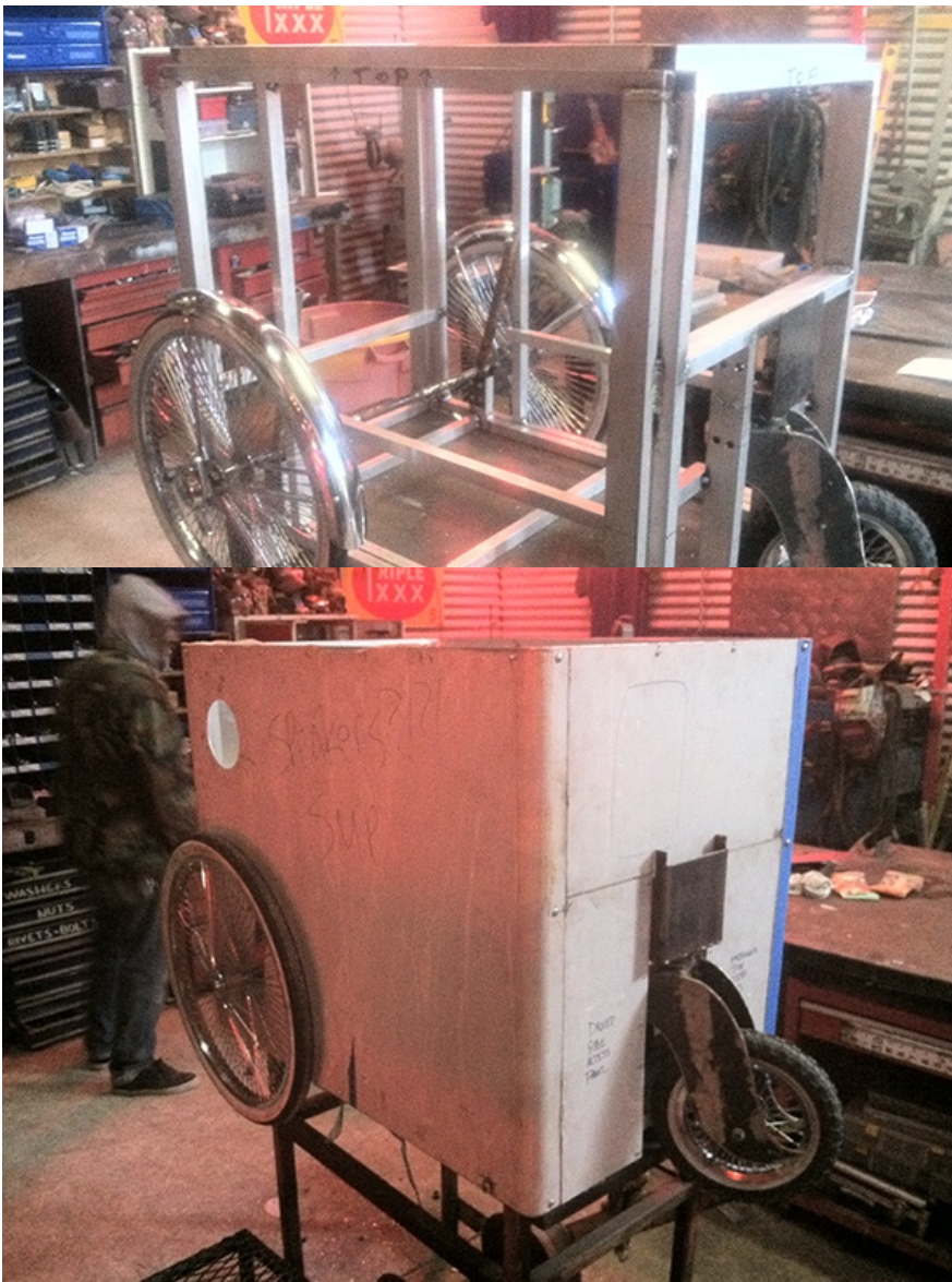
Figure 24 Paleta cart with insulation and outer walls
