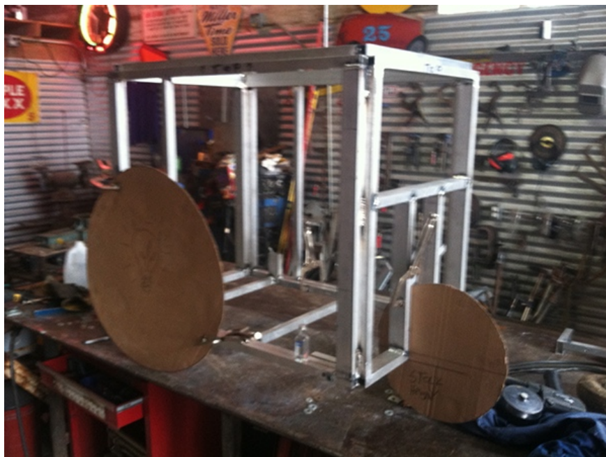
Figure 22 Paleta cart frame with cardboard wheels, a prototype
