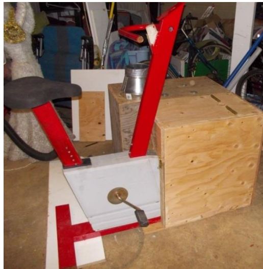
Figure 5-4 Bicycle Attached to Blower Box
