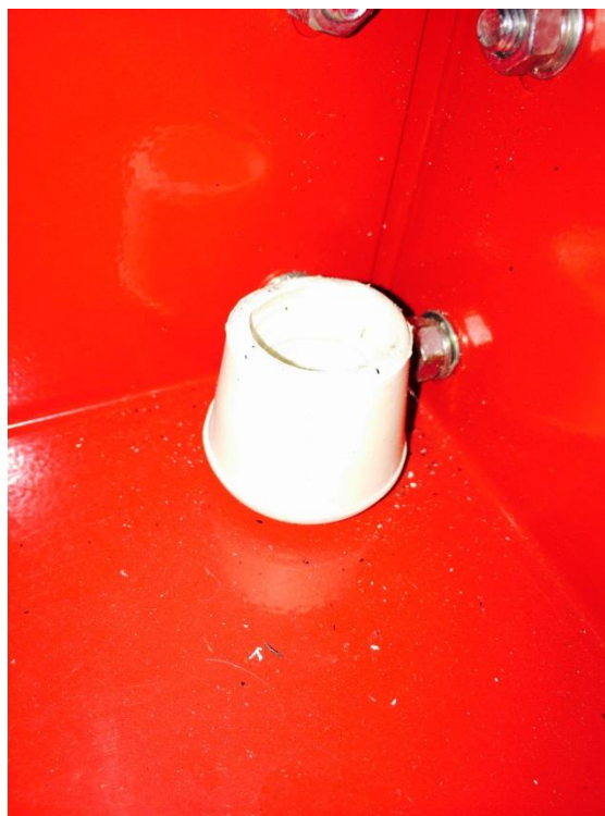
Figure 5-6 Rubber Feet used to mount the top structure to the tool cart
