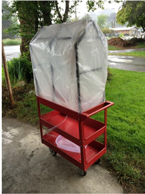
Figure 5-3 Top Structure with the cover attached
