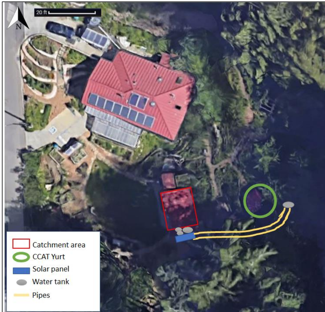
Figure 1. Aerial map of the Campus Center for Appropriate Technology (CCAT) Rainwater Catchment & Solar Water Pump system. The long pipes (yellow) are partially underground.
