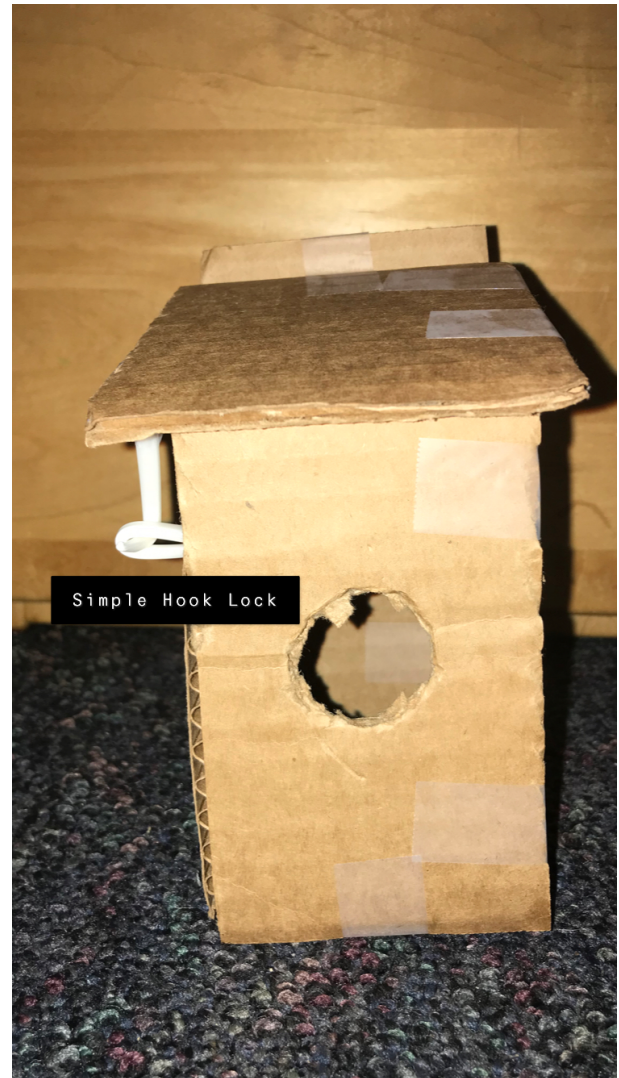
Figure 5-8: Prototype of side hinge as an opening method. Built and photographed by Rize Martins de Oliveira
