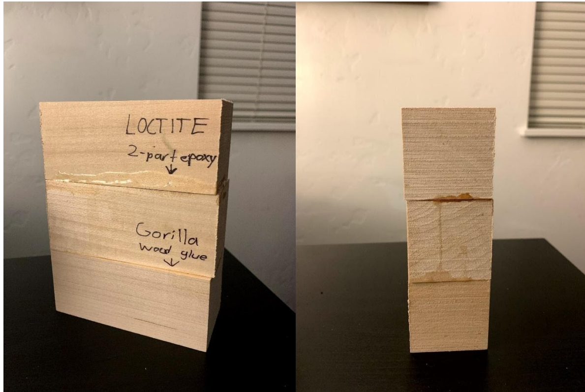
Figure 5-10: Adhesive test done to visually compare and test waterproofness between LOCTITE epoxy and Gorilla wood glue. Test conducted and photographed by Alex Garza
