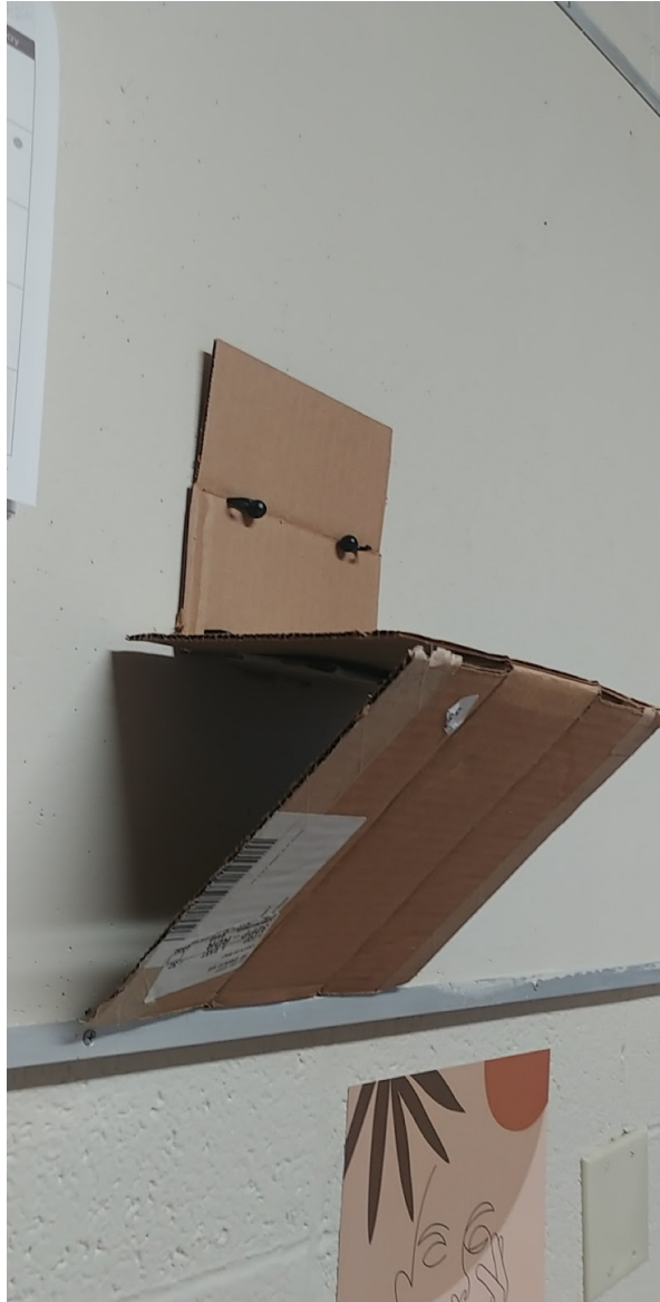
Figure 5-5: Prototype of wall mounting method with support strip. Built and photographed by Valerie Keody
