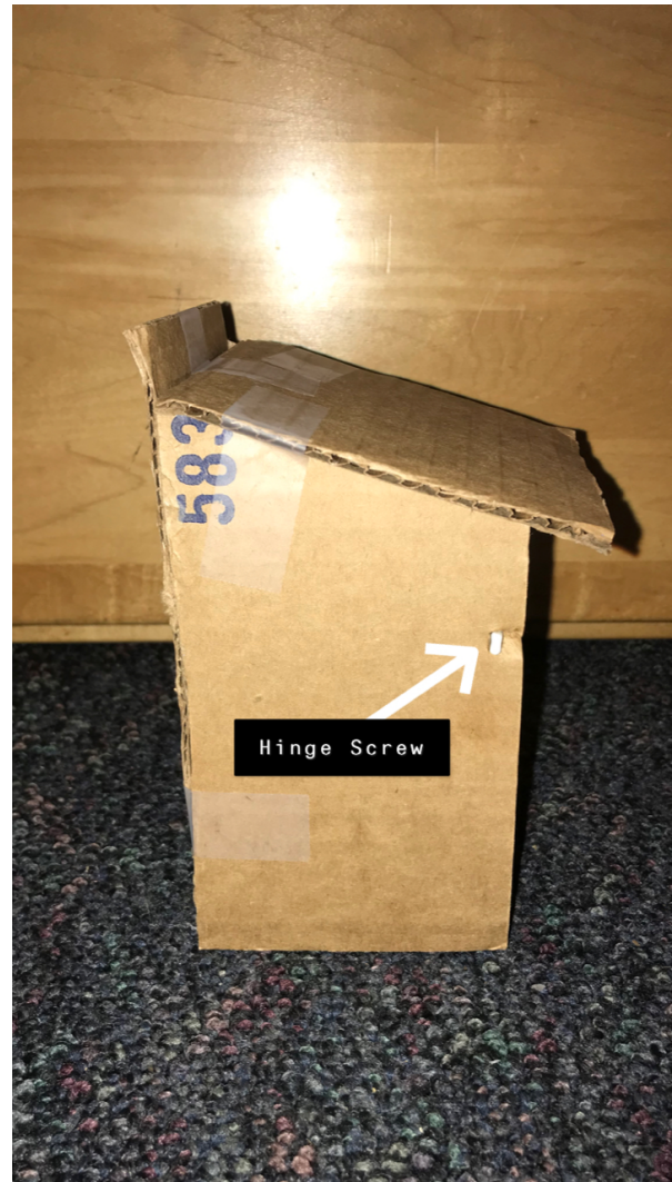
Figure 5-7: Prototype of revolving front panel as an opening method. Built and photographed by Rize Martins de Oliveira
