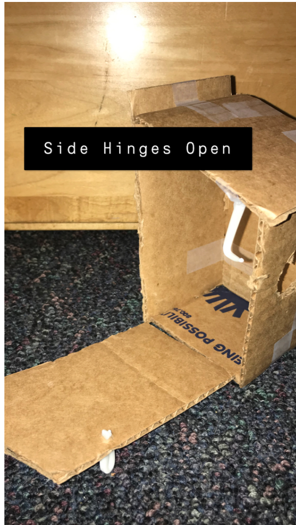
Figure 5-8: Prototype of side hinge as an opening method. Built and photographed by Rize Martins de Oliveira
