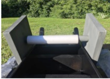
Figure 5.6.1: Wooden Dowel inside PVC Pipe attached to squares with screws
