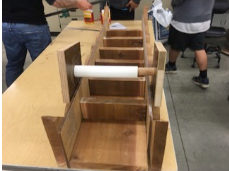
Figure 5.6.4: Inside track sandwiched between baseboards and outside track, screwed in with 3- inch screws
