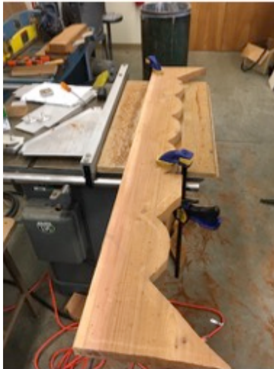
Figure 5.6.2: Traced out and cut track, bottom on left and top on right
