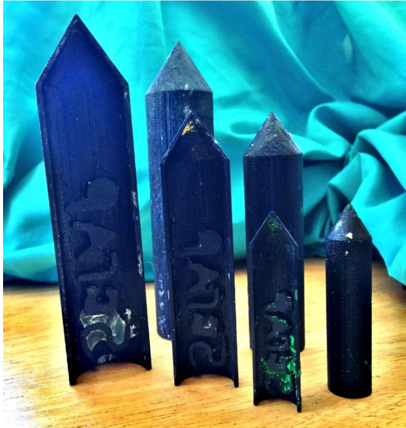
Figure 5-3: 3-D printed molds for both candles and crayons designed by team SuperStar.
