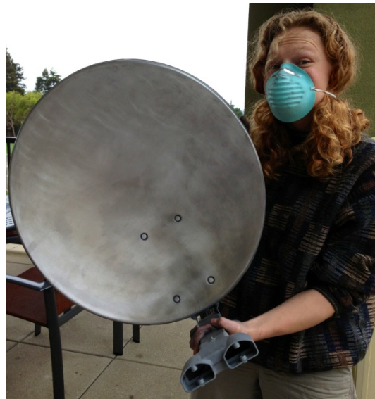
Figure 52 Sanding a DISH satellite to expose the reflective metal surface (respiratory and eye protection required).
