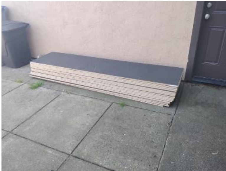
Figure 5-3 MDF material used to build the cubbies. (Robert Carey)
