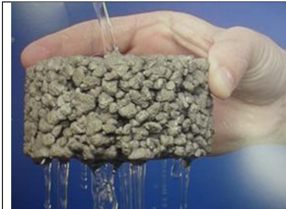
Figure 12: A demonstration of pervious concrete (Image Source: http://www.nebrconcagg.com/pervious.html )
